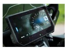
With a screen size and resolution that can be customized to suit OEM requirements, this compact Bluetooth-enabled unit combines a broad range of information and communication functions in a single device. Innovative features like OS-independent mySPIN smartphone integration can be utilized thanks to the built-in Wi-Fi connectivity. Optical bonding and an anti-reflection coating ensure enhanced screen readability, even in strong sunlight.
