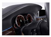
The 12.3" digital instrument cluster with IPS display was the first cluster with Full HD resolution (1920 x 720 pixels) on the market. The cluster is optically bonded and ensures – in combination with an anti-glare and anti-reflection coating – a higher ambient contrast and improved readability due to reduced light refraction. The cluster is an impressive package that exudes quality and combines ruggedness with an enhanced look and feel
